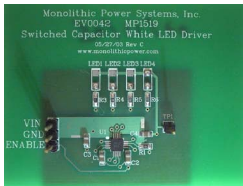
Figure 1: EV0042 Evaluation Board
